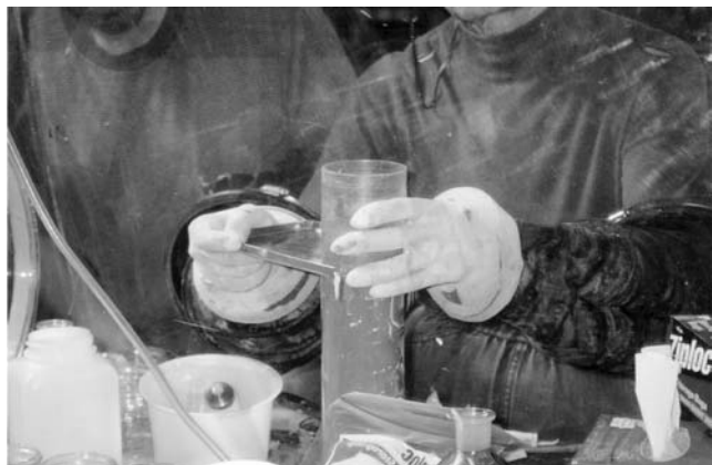
Figure 1. Photograph of sample sectioning for transferring to a storage vessel, using a deoxygenated glovebox
